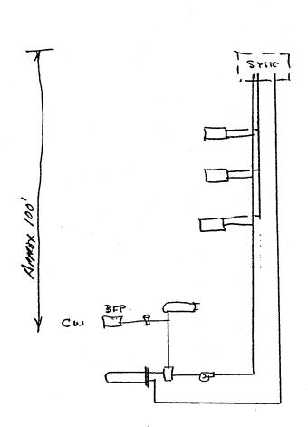
System Pressur 50 psi (115') Pump head = (40')
